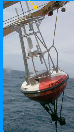
Moored Surface Buoy
